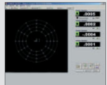
Plane5 — Project Setup Screen. Configure shape and # of points for up to 7 surfaces.
